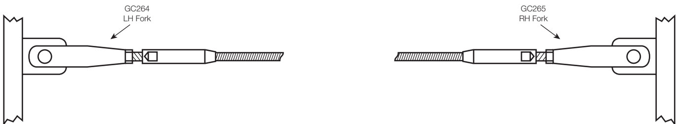
System 8: Left and right hand adjustable forks for connection to welded lugs
